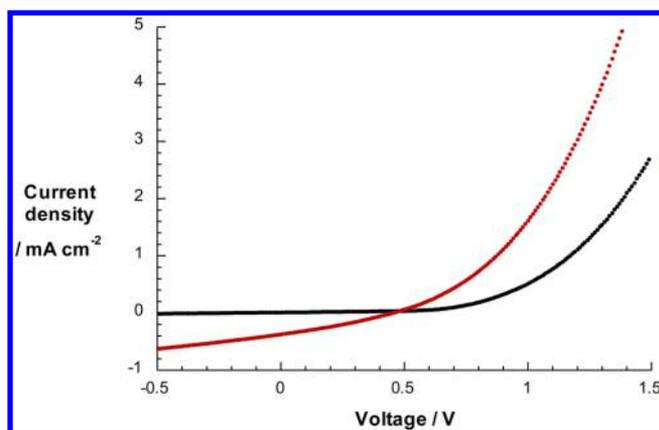
**Figure 9.** Current density–voltage ( $J$ – $V$ ) characteristics—a short circuit current density ( $J_{SC}$ ) of 0.38 mA, an open circuit voltage ( $V_{OC}$ ) of 0.46 V, a fill factor (FF) of 30.24%, and an efficiency ( $\eta$ ) of 0.054%—under AM 1.5 radiation with the illuminated current density and dark current density shown as red and black lines, respectively.
